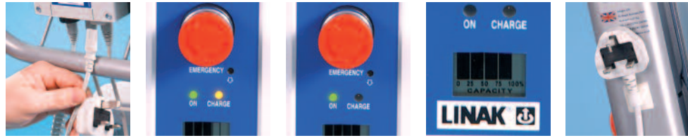
Fig 1 Fitting / removing mains lead to / from control box Fig 2 Image showing the green power 'ON' light and the amber 'CHARGE' light Fig 3 Image showing the green power 'ON' light and the 'CHARGE' light out. Fig 4 Image showing the battery level indicator showing 4 bars Fig 5 Image showing the mains lead plug mounted on the hoist.
